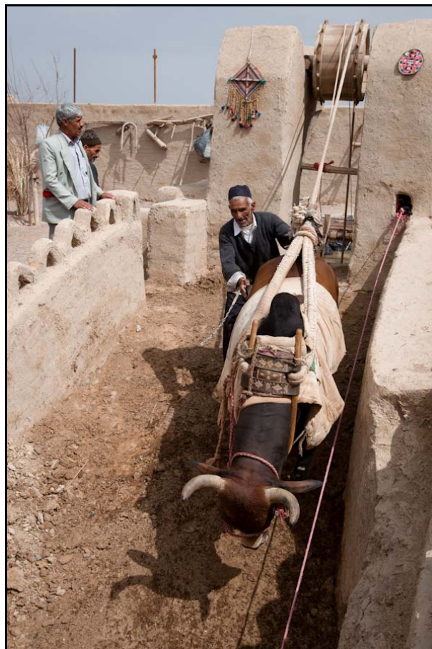
Figure 106: Water being lifted from a Zajara well using oxen in central Iran
