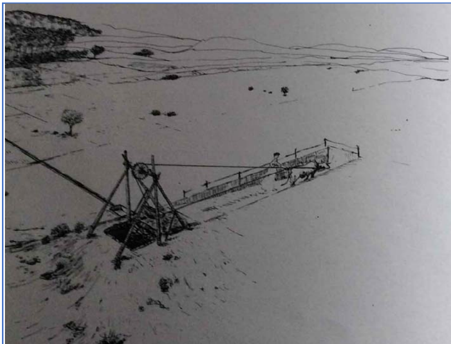
Figure 103: An illustration of a wooden Zajara well in use on the coastal Batinah plain in Oman (Costa and Wilkinson 1987, 40, Fig. 6)
